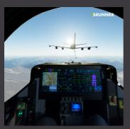
To reach training perfection BRUNNER has resembled a proper F-35 replica cockpit, BRUNNER control loading devices and the Aechalon IG on the well known NOVASIM platform. In a Mixed Reality trainer, the authenticity of the replica cockpit is essential.
