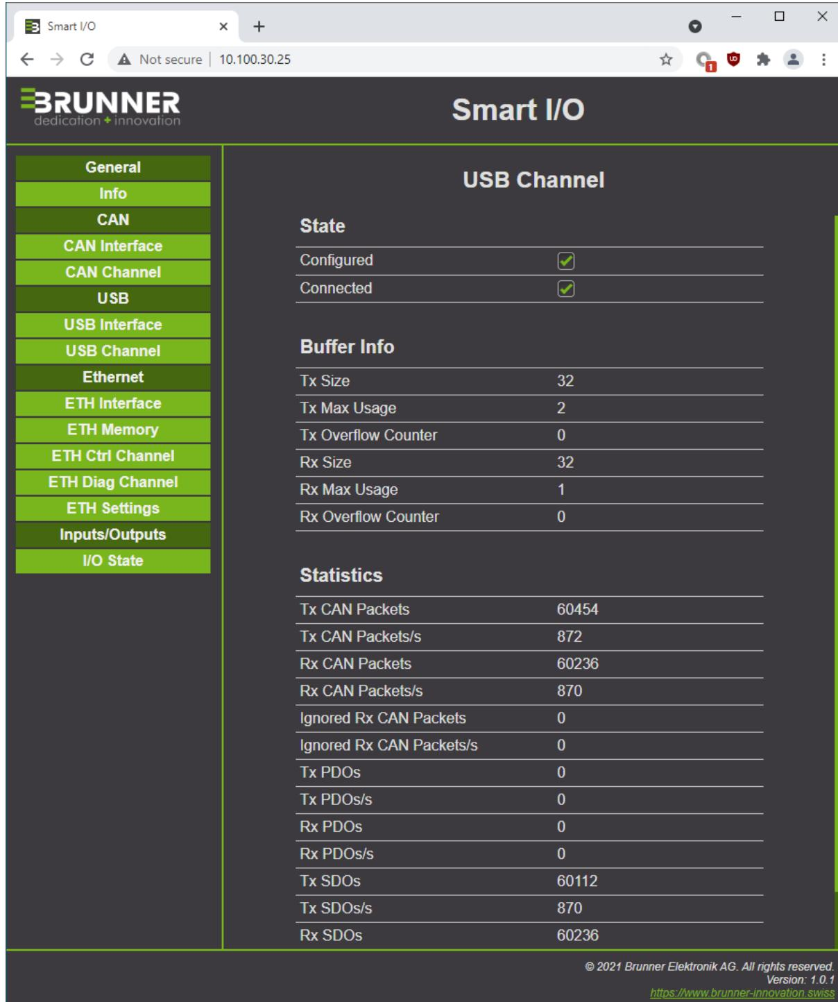
The screenshot shows a web browser window titled "Smart I/O" with the URL "10.100.30.25". The left sidebar menu includes: General, Info, CAN, CAN Interface, CAN Channel, USB, USB Interface, USB Channel, Ethernet, ETH Interface, ETH Memory, ETH Ctrl Channel, ETH Diag Channel, ETH Settings, Inputs/Outputs, and I/O State. The main content area is titled "USB Channel". It contains three sections: "State", "Buffer Info", and "Statistics".
