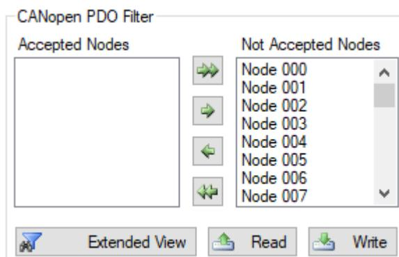
The PDOs of the nodes listed in “Not Accepted Nodes” won’t be routed through the gateway. This is typically used when the CAN traffic is monitored, but certain process data isn’t of interest.
